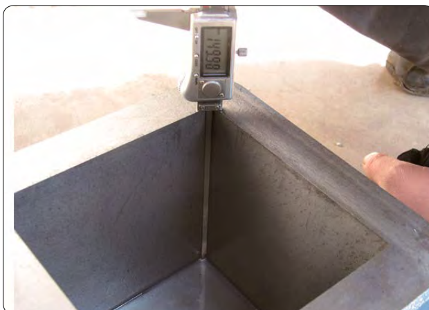
Verification of dimension using electronic digital display depth caliper
