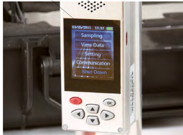
Detail of HT-225W Concrete test hammer
