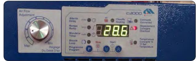
Control panel and air flow adjustment knob
