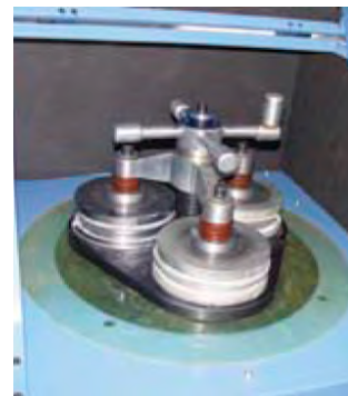
Internal clamping part for model ZHM-3B
