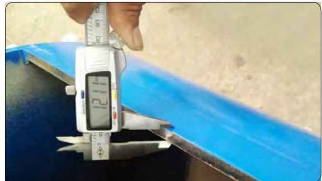
42-5305/01 Los angeles abrasion machine with 12mm wall thickness
