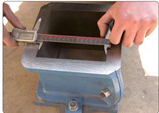
Verification of dimension using digital vernier caliper
